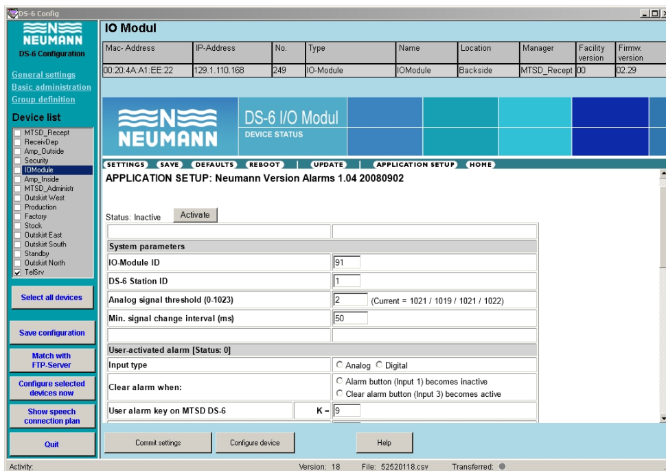
Figure: Configuration of the I/O Module by DS-6 Config
